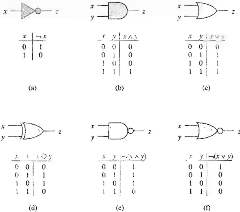
**Figure 29.1** Six basic logic gates, with binary inputs and outputs. Under each gate is the truth table that describes the gate's operation. (a) The NOT gate. (b) The AND gate. (c) The OR gate. (d) The XOR (exclusive-OR) gate. (e) The NAND (NOT-AND) gate. (f) The NOR (NOT-OR) gate.
