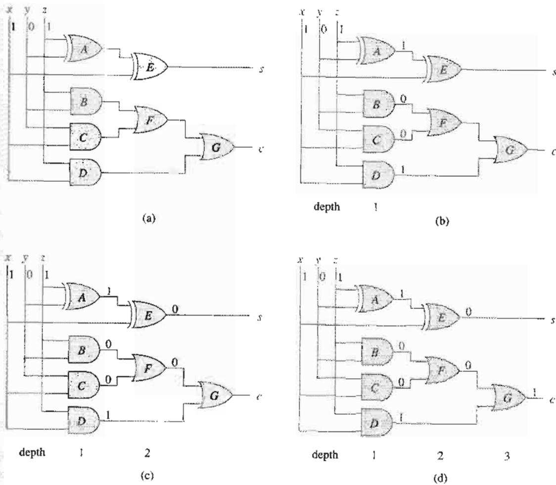
**Figure 29.2** A full-adder circuit. (a) At time 0, the input bits shown appear on the three input wires. (b) At time 1, the values shown appear on the outputs of gates  $A$ – $D$ , which are at depth 1. (c) At time 2, the values shown appear on the outputs of gates  $E$  and  $F$ , at depth 2. (d) At time 3, gate  $G$  produces its output, which is also the circuit output.
