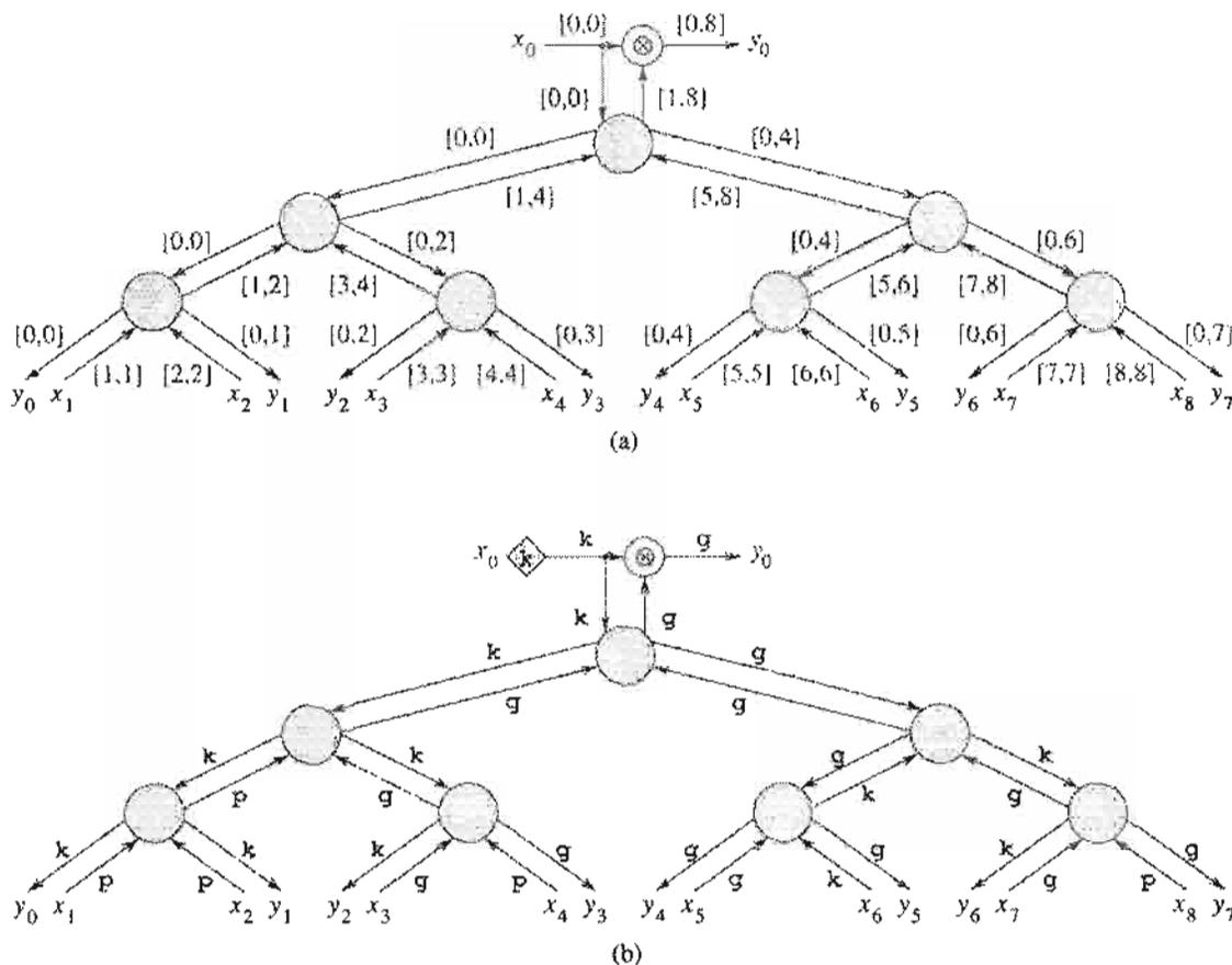
**Figure 29.9** A parallel prefix circuit for  $n = 8$ . (a) The overall structure of the circuit, and the values carried on each wire. (b) The same circuit with values corresponding to Figures 29.3 and 29.7.
