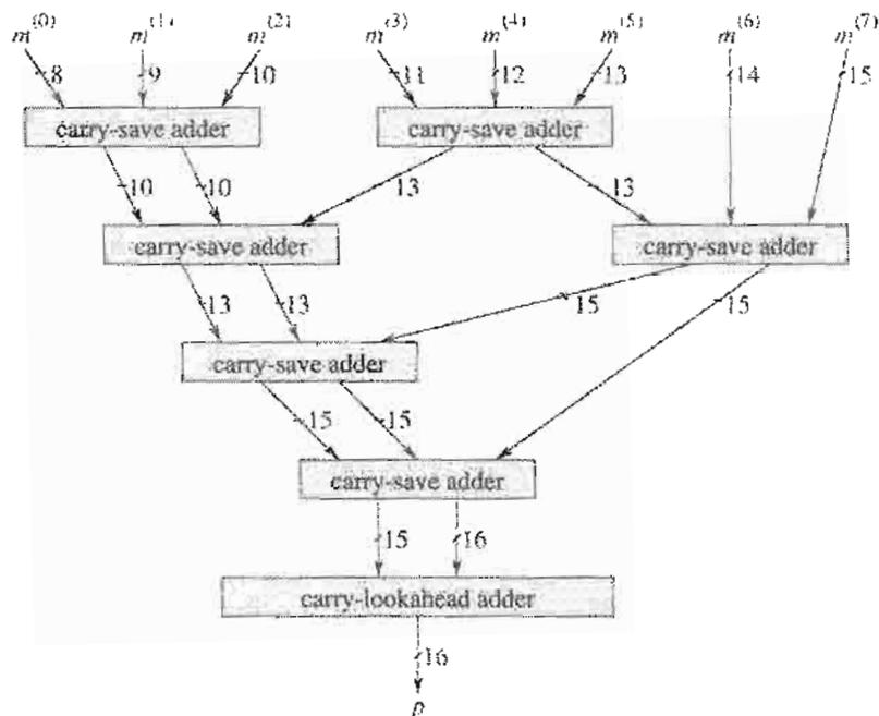
**Figure 29.16** A Wallace tree that adds  $n = 8$  partial products  $m^{(0)}, m^{(1)}, \dots, m^{(7)}$ . Each line represents a number with the number of bits indicated. The left output of each carry-save adder represents the sum bits, and the right output represents the carry bits.
