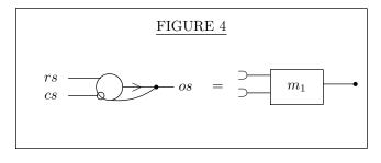
It should be noted that this  $m_1$  corresponds to the actual vacuum tube trigger circuits mentioned at the beginning of 5.1. It is worth mentioning that  $m_1$  contains one E-element, while the simplest trigger circuits contain one or two vacuum tubes (cf. loc. cit.), in agreement with the estimates of 6.5.
