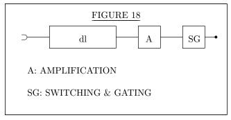
dl is to be used as a memory its output must be fed back—directly or indirectly—into its input. In an aggregate of many dl organs—which M is going to be—we have a choice to feed each dl back into itself, or to have longer cycles of dl 's: Figure 19 (a) and (b), respectively.
