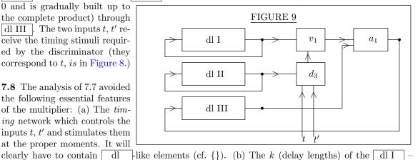
dl III . These too have certain functions of synchronization: Each time when the adder functions (that is in each interval it-ft) the multiplicand and the partial product sum (that is the outputs of dl I and of dl III ) must be brought together in such a manner that the former is advanced by t (moved by one position to the right) relatively to the latter, in comparison with their preceding encounter.
