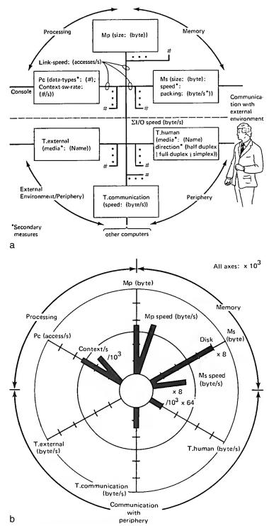
Figure 2. Transformation of structure summary into performance summary. (a) PMS diagram redrawn. Note components as boxes. (b) Major components of PMS diagram form the six major axes of performance: processing, primary and secondary memory, communication to humans or other computers (e.g. a network), and the computer's peripherals from *Computer Structures* (1982).<sup>2</sup>
