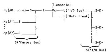
Figure 1. A simplified PMS diagram of the DEC PDP-8 from *Computer Structures* (1971).<sup>2</sup> Note the components without boxes. PMS diagrams can reveal exceptional detail, including all the linking busses, controllers, and so forth, and especially all the component specifications.
