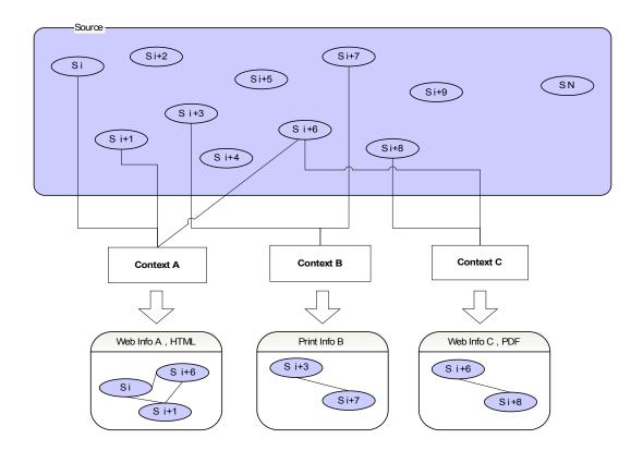
In the above diagram, content objects (Si, ..., Si+n) are free-floating objects in the Source area. Topics are collected into Contexts (A, B, C, ...) and point to sets of content objects. Each Context has different targets (Web, Print, etc.).
