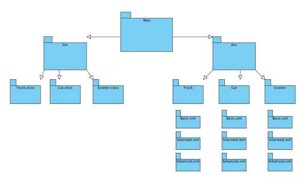
The above diagram shows an example of how folder structure should be created. The example is to have three Java objects compiled out to the bin folders, Truck.java, Car.java, and Scooter.java, and we want to create document files and map them to these class objects.
