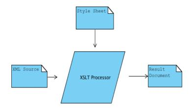
The transformation process occurs as in the above diagram. First, the XSLT processor parser reads the input XML source and parses it into a tree. With the style sheet as the second input, the engine transforms the tree by using the transformation template rule which is defined in the style sheet. Finally, the serializer writes the result tree out to the result document.
