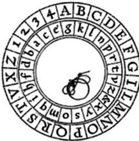
Figure 2. An Alberti cipher.
