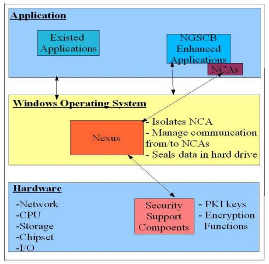
This diagram shows the interaction between applications, operating systems, and hardware device
