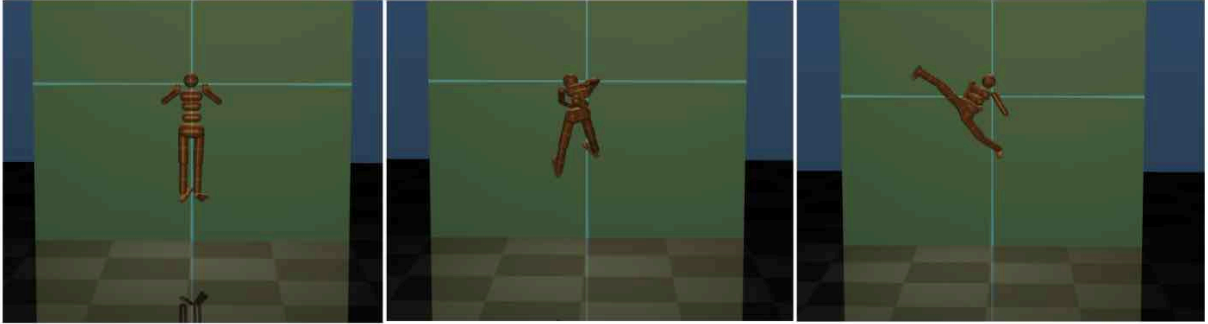
Figure 11: Simulation images after training humanoid-RockClimb using DDPG for 1M time-steps
