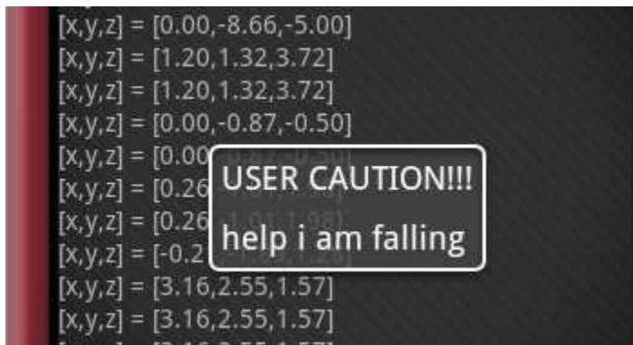
Fig 8.1: The alert message when phone starts falling and accelerometer values being recorded.
