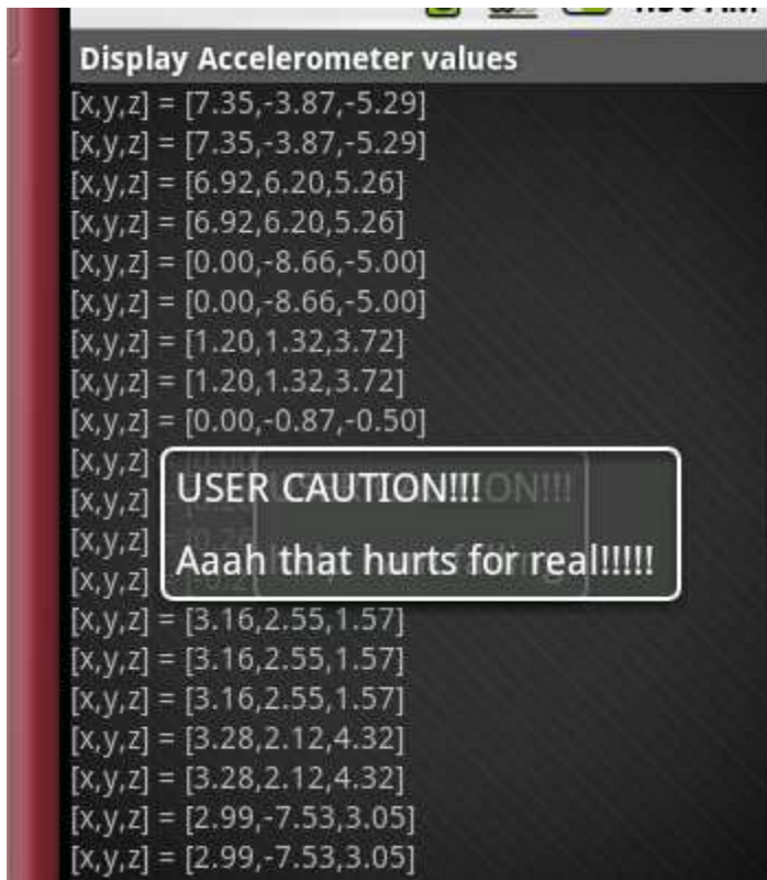
Fig 8. The UI screen with accelerometer values and alert message when the phone has reached ground.
