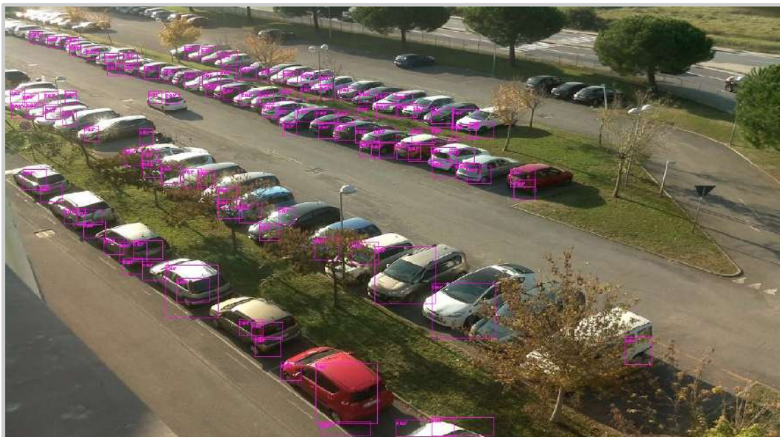
Figure 11: Poor detection with fixed camera angle. There are too many false positives with the threshold so low (5% in this case). At higher thresholds, few or none of the cars are correctly identified.
