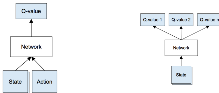
(a) Naive formulation of deep Q-network (b) Optimized architecture of deep Q-network
