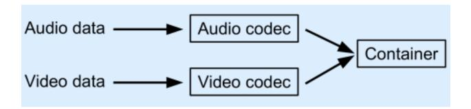
Playback of a multimedia file operates in the exact opposite direction.. Once the container used is identified, it tells us which codecs are needed to decode the data. The audio and video
