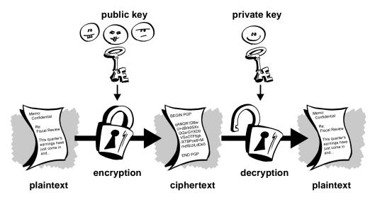
Figure 2-1. Public Key Cryptography diagram
